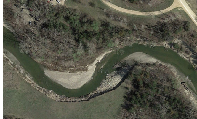
Fig. 1. Bedload originating from eroding streambanks is often deposited in channel immediately downstream of the eroding outer bend.
