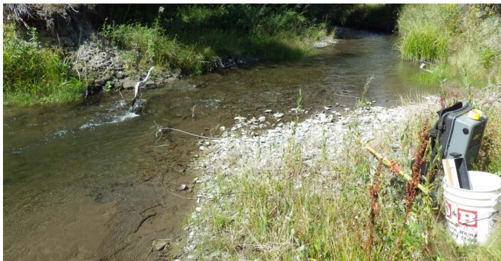
Pre-positioned aerial electrofishing setup with wire-loop anode in Trapper Creek. Credit: D. Dauwalter.
