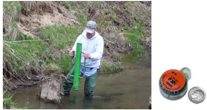
Fig. 7. Deploying a logger (right) for continuous measurement of water temperature at a stream restoration monitoring site.
