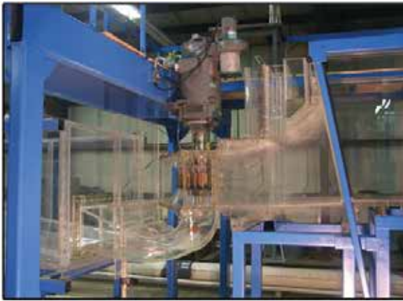
Figure 1. Left: U.S. Army Corps of Engineers Engineering Research and Development Center (ERDC) hydraulic observational turbine model (1:25 scale) for the Ice Harbor runner replacement project. Photo credit: USACE. Right: Computational fluid dynamics (CFD) model used to predict the probability of fish passage through various regions of the turbine. Photo credit: USACE.
