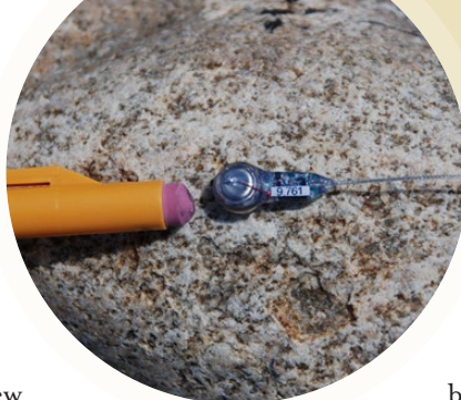
Radio telemetry tag: a small but powerful tool for tracking fish.
