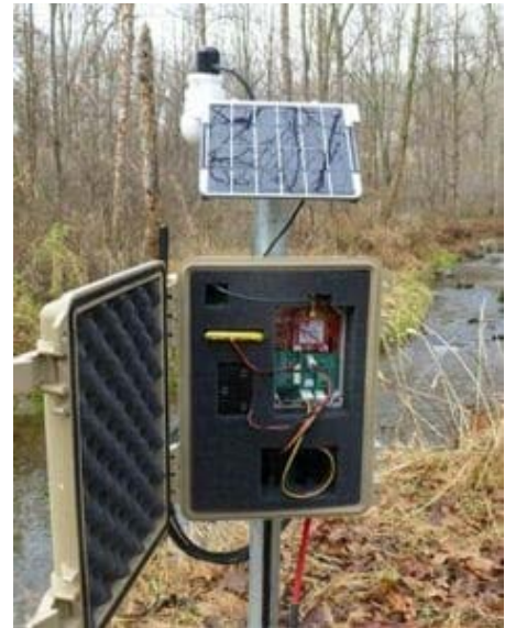
Figure 5. A DIY Mayfly water quality monitoring station deployed by Trout Unlimited.
