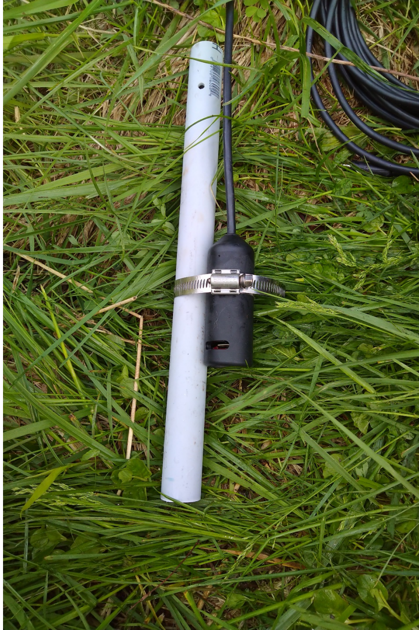
Figure 12: Attach sensor to PVC with large hose clamp.
