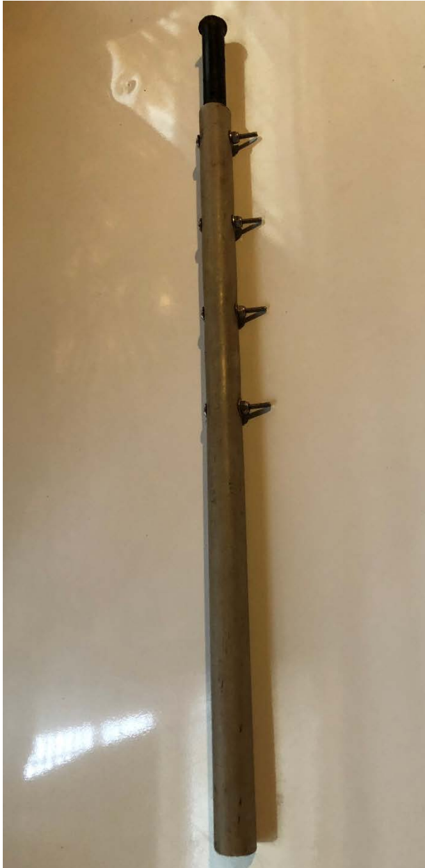
Figure 5: To create extension rod, drill 3 or 4 holes in PVC that line up with pre-drilled holes on a 24 inch steel rebar pin. Cut PVC so that the steel rebar pin extends approximately 3-4 inches above the top of the PVC, and the PVC extends 2 inches below the steel rebar pin (this helps keep the extension rod on another rebar piece when pounding it into the streambed). Attach the pvc using appropriately sized bolts, washers and nylon lock nuts.
