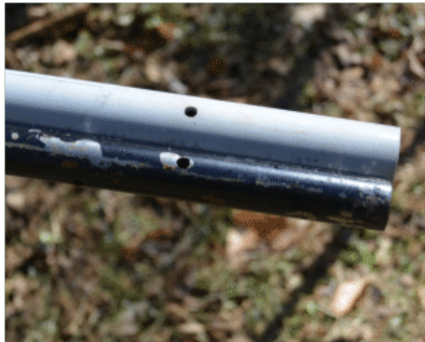
Figure 7: Lining up retaining pin holes
