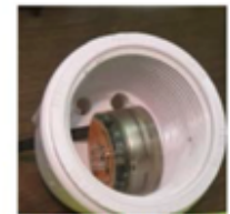
FIGURE 7. TIDBIT FASTENED INTO PVC CAP USING A TIE STRAP (ZIP TIE).
