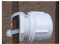
FIGURE 8. PVC HOUSING FIXED TO REBAR USING A NYLON STRAP (ZIP TIE).
