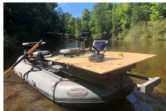
Thermal imaging surveys are often conducted from our raft. The plywood panel serves as a landing pad when suitable landing zones are not available nearby.
